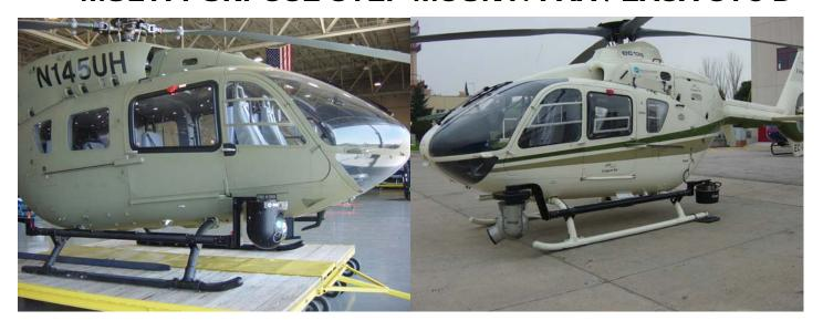
The step mount expands the capability of both the EC-135 and EC-145 models. Available in left / right and lightweight original step replacement versions, the step mount is the most capable and cost effective method of installing all the most popular sensors on these airframes
